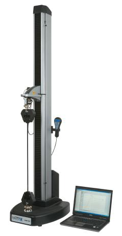
The LS2.5 is a 2.5 kN / 562 lbf high precision material testing machine that combined with our extensive range of grips, fixtures, extensometers and software creates a powerful material testing system. The system is equally suited to quality control, educational and R&D environments within a wide range of applications and test types. The system is particularly suited for plastic, rubber and other high elongation materials due to its wide crosshead travel capability.
